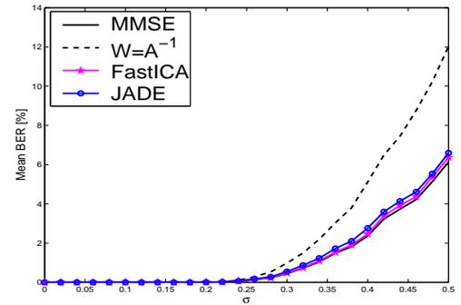
**Fig. 1.** Mean bit error rate of separated BPSK signals in noisy environment with  $\mathbf{A} = \begin{pmatrix} 1 & 1 \\ 1 & 0.2 \end{pmatrix}$  computed from 100 trials for each  $\sigma \in [0, 0.5]$ . MMSE solution is much proper than that minimizing SIR (4), i.e. inversion of  $\mathbf{A}$ .
