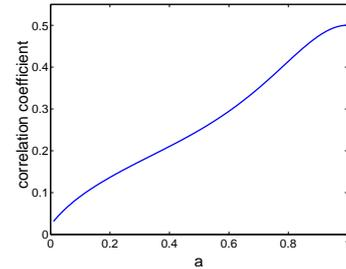
**Fig. 3.** Correlation coefficient of two MMSE components when  $\sigma = 0.3$  for mixing matrix  $\mathbf{A} = \begin{pmatrix} a & a \\ 1 & a \end{pmatrix}$  with varying parameter  $a \in [0, 1]$ . Matrix  $\mathbf{A}$  is singular for  $a = 0, 1$ .
