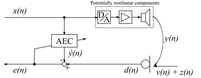
Fig. 1. The process of Acoustic Echo Cancellation
