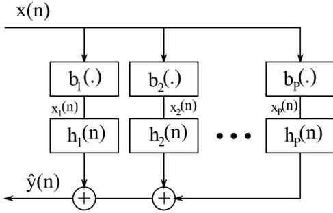
Fig. 3. The structure of the proposed power filter
